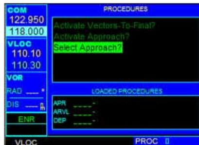
3. A window appears listing the available procedures. Turn the large right knob to highlight the desired procedure and press the ENT Key.
