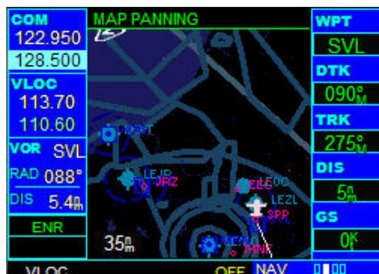
Another Map Page function is panning, which allows the map to move beyond its current limits without adjusting the map. When the panning function is selected (by
