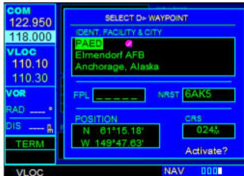
2. Use the small and large right knobs to enter the identifier of the desired destination waypoint.
