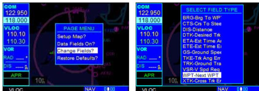
'Change Fields?' allows selection of the data displayed on the four user-selectable data fields along the righthand side of the Map Page. There are twelve available data types, as described in DEFAULT NAV PAGE above. Refer to that section to see how to change the fields.
