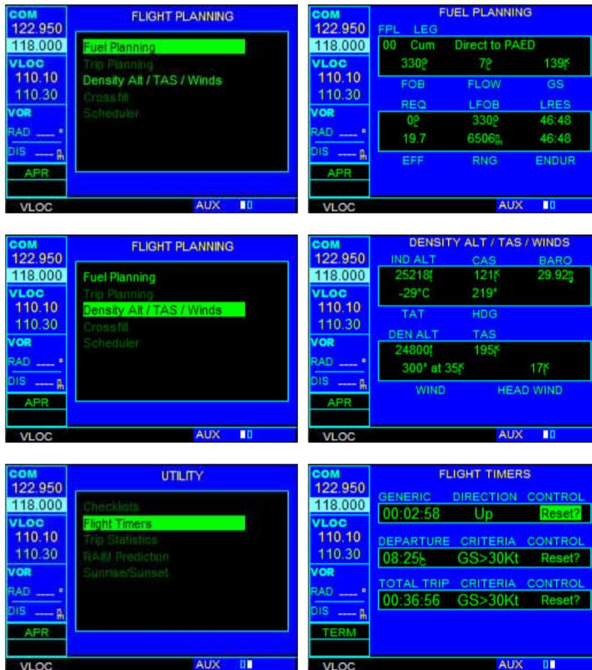
The AUX pages also provide functions such as fuel planning, density altitude, true airspeed, and winds aloft calculations
