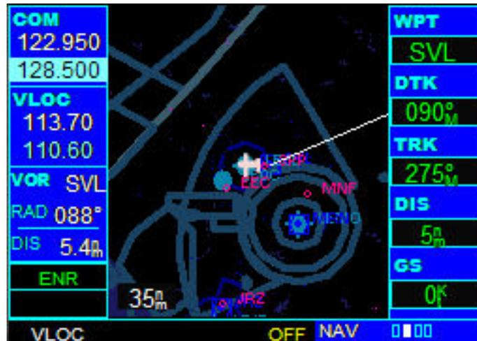
At the right of the MAP Page there are user-definable fields which display the data needed as the flight progresses. By default these fields display: Next Waypoint (WPT), desired track (DTK), ground track (TRK), distance to destination (DIS) and ground speed (GS). However, each of these fields can be customized to display a different data item. Available data items include:
