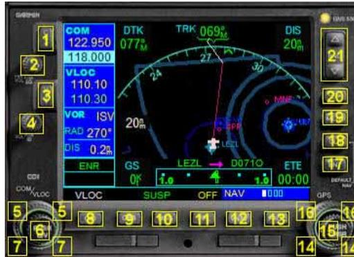
1. The COM Flip-flop Key is used to swap the active and standby COM frequencies.
