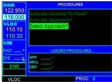
The Procedures Page is displayed by pressing the PROC Key. The Procedures Page provides direct access to approaches based upon the active flight plan or direct-to destination. In either case, the departure and destination airports must have published procedures associated with them.
