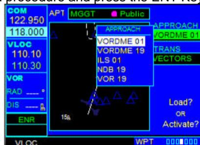
4. A second window appears listing the available transitions. Turn the large right knob to highlight the desired transition waypoint and press the ENT Key. (The approach 'Vectors' option assumes the pilot will receive vectors to the final course segment of the approach and will provide navigation guidance relative to the final approach course.)
