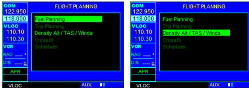
The Flight Planning Page provides access (via 'menu options') to functions for fuel planning and density altitude/true airspeed/winds aloft calculations. When a menu option is selected, the corresponding page appears providing additional information.
