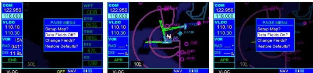
The 'Data Fields Off?' option provides a full-screen Map Display, without the five data fields along the right-hand side of the screen. Select this option to display a larger map area. If this option has been selected and the data fields are off, 'Data Fields On?' appears as an option instead in the page menu.
