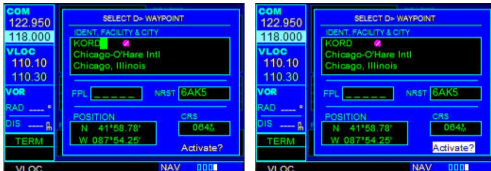
3. Press the ENT Key to confirm the selected waypoint, and press the ENT Key again to activate the direct-to function.
