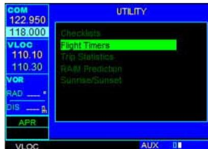
The Utility Page provides access (via 'menu options') to Flight Timers which leads to Flight Timers Page.
