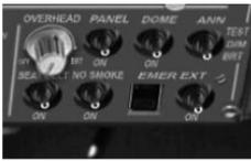
Here you'll find the switches for the Cabin Signals „Seat Belts“ and „No Smoking“ as well as the switches for the Panel Lights.
