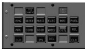
The button T/O CONFIG fulfills the following function: it simulates the TO/GA situation, to make sure that all systems are ready for take off. This test needs to be done during the Take-Off Checklist before the start.
