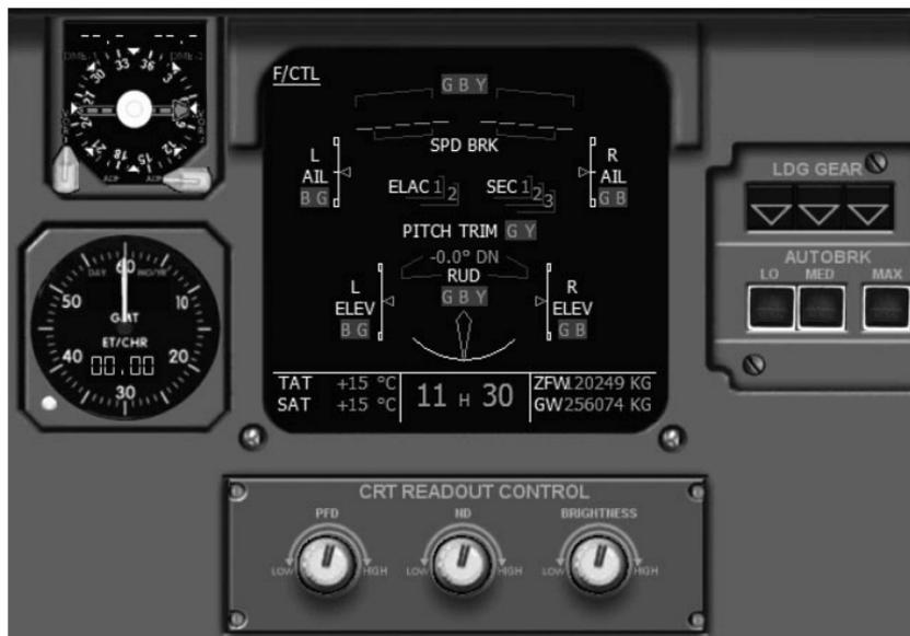
Here you'll find the complete System Display (SD). The SD displays information for all the various aircraft systems. The displayed information changes automatically according to the actual flight situation.
