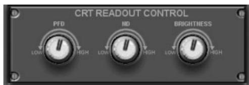
All the three knobs can be operated with the help of the mouse. The left knob dims the Primary Flight Displays (PFD). The center knob dims the Navigation Displays (ND). The right knob dims all four displays and the FMGC together.
