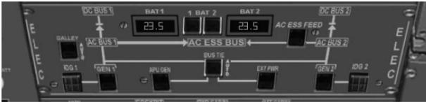
This part of the panel holds the Battery Switches. In reality this aircraft has two independently working batteries. Flight simulator though, only recognizes one battery.
