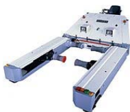
Power Push Unit, designed to be attached on one of the main landing gear.
