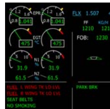
E/WD layout on an old-generation panel with EPR logic (such as an A320 equipped with IAE engines).
