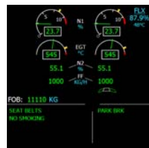
E/WD layout on a new-generation panel with N1 logic (such as an A318 equipped with CFM56 engines).
