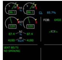
Typical E/WD layout on an old-generation panel with N1 logic (such as an A320 equipped with CFM56 engines).
