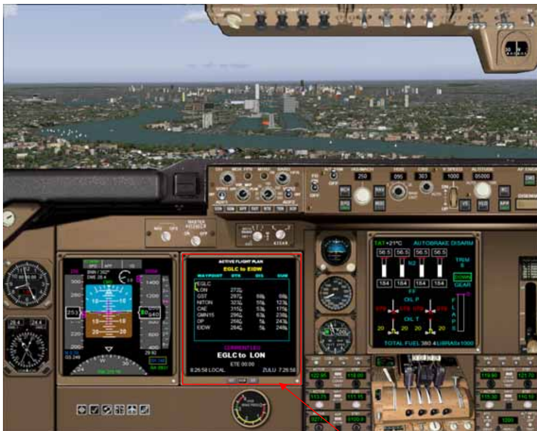
MFD screen mode Flight Plan list
