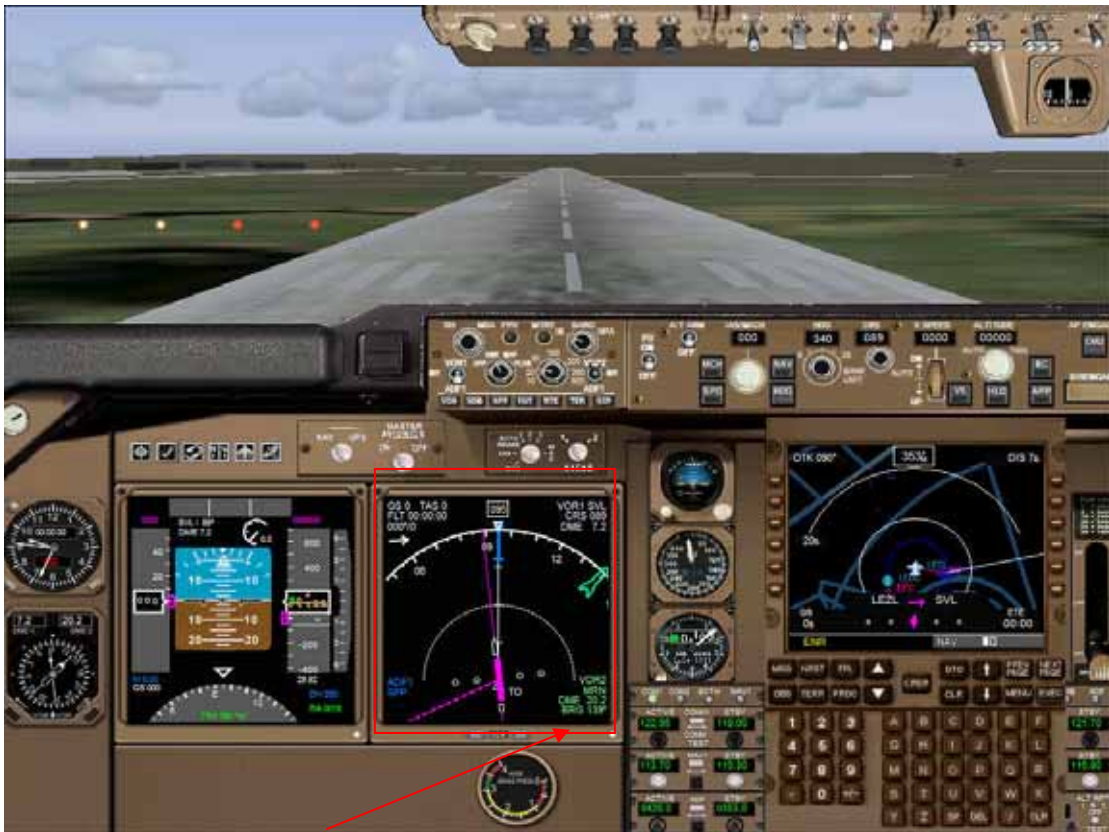
MFD screen mode MAP. New GPS FMC style.
