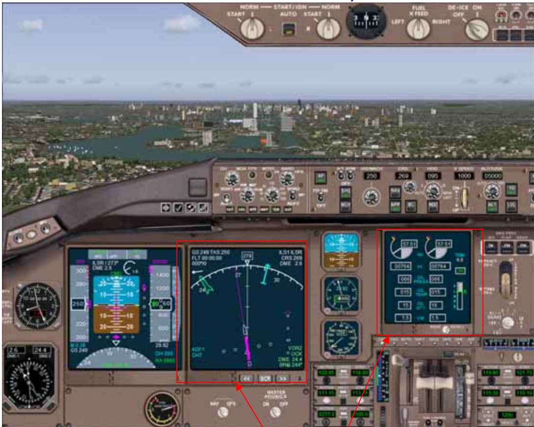
MFD screen mode arc APP ARC, EICAS 2
