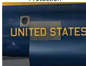
APU Exhaust Heat-Protection
