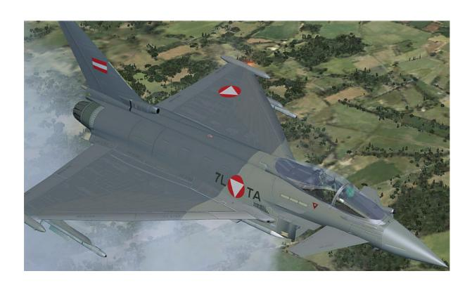
With the Eurofighter Typhoon, in subsonic flight the pressure point lies in front of the centre of gravity, therefore making the aircraft aerodynamically unstable, and is why Eurofighter Typhoon has such a complex Flight Control System – computers react quicker than a pilot.
