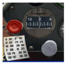
These cards are normally near the compass, but in FS that is hard to do. To steer by the magnetic compass, just make sure the aircraft is stable and not changing speed and look at the chart below. If you need to fly 150° degrees, steer 147° on the compass.
