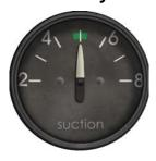
The vacuum system drives the Gyro Compass (Direction Indicator) and the Artificial Horizon (Attitude Indicator). The low pressure is generated by en engine driven pump and you will be able to monitor the pressure on the Suction Gauge. Normally you will see pressures around 5. When lower values are indicated the vacuum driven instruments will not function reliable. A probably cause is most probably a leaking flexible hose or blocked inlet filter.
