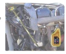
pressure to drop and engine temperature to be higher then normal. Apart from reducing power and diverting to the nearest airport there is little that can be done. The engine needs oil to operate. Now will you take the pre flight checklists serious?
