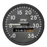
There are a lot of pilots who do not fully understand the operation of direct drive, fixed pitch, normally aspirated engines. When they climb to thinner air they tend to see the RPM climb get close to the take-off RPM and are tempted not to lean the mixture to reduce RPM. But because of the fixed pitch propeller and the thinner air you will NEED those high RPM to get your cruise power. Do not fear high RPM as long as you stay under the maximum allowed RPM. One more reason to stay low!
