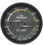
The oil pump will pressurize the oil system and the pressure is indicated by the oil pressure gauge. Oil pressure should be between 60 and 85 PSI and this has to be achieved in 30 seconds after engine start. Oil temperature is also indicated by the same gauge and should be between 100°F and 240°F. Please note that the Super Cub has no warning lights for oil pressure, you will need to keep track of it.
