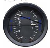
The Cylinder Head Temperature / Exhaust Gas Temperature help you determine if the fuel/air ratio is correct. The CHT measures the temperature of the sparkplug and the EGT measures the temperature a few inches from the cylinder. Thus the EGT will always be a bit faster in changing as there is no mass to warm or cool.
